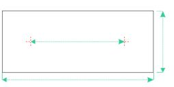
Since it is an elastic fabric, here the approx. standard dimensions: 60 x 25 mm, Standard pitch hole approx. 40 mm
